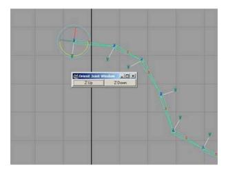
Now simply select your joints one at a time and press either Z-up or Z-down to make all of your local rotation axis point in the same direction. Note this script points the Y-Axis toward the next joint.
