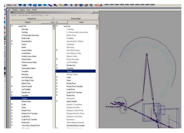
Group the controller to itself and parent the group to the "neckMid" joint. freeze transform on the controller...
