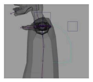
Now you want to move the curve in line with the spine from the front of the character and then snap the pivot of the curve to the "low\_upperSpine" joint.
